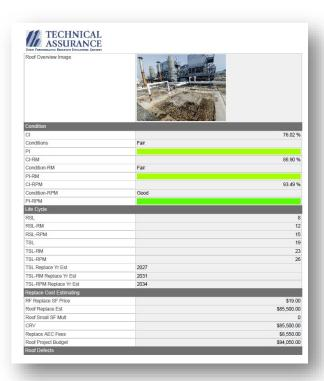
The inventory and assessment data was collected using the ON-PNT® mobile field app. Our team performed (and repaired) core cuts in order to determine the full roof system make up and to verify wet roof areas.
